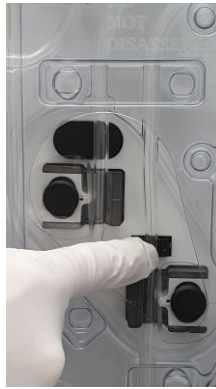
Figure 12: Fibre IN sensor tubing installation
