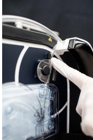
Figure 22: Reinfusion line presence sensor
