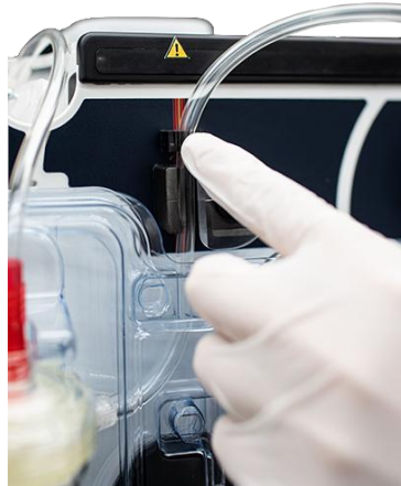
Figure 23: Waste sensor tubing installation
