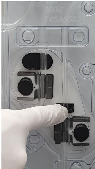
Figure 63 : Installation tubulure capteur Fibre IN
