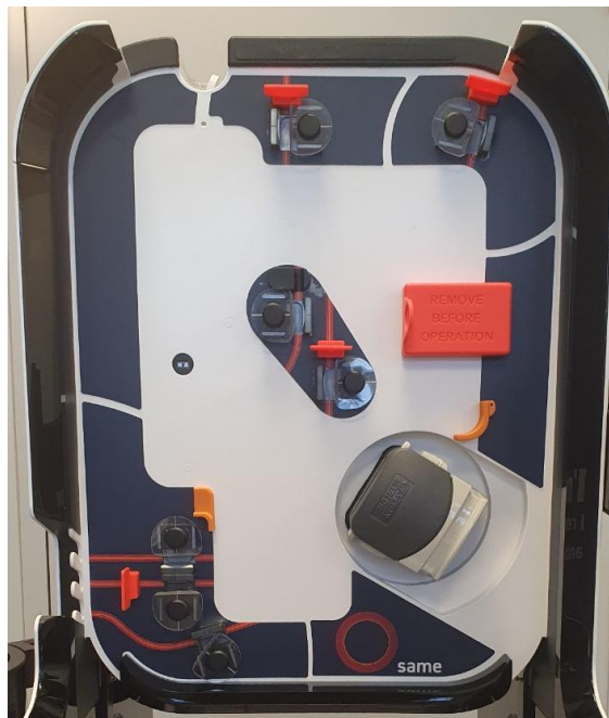
Figure 31: Covers protecting the optical sensors
