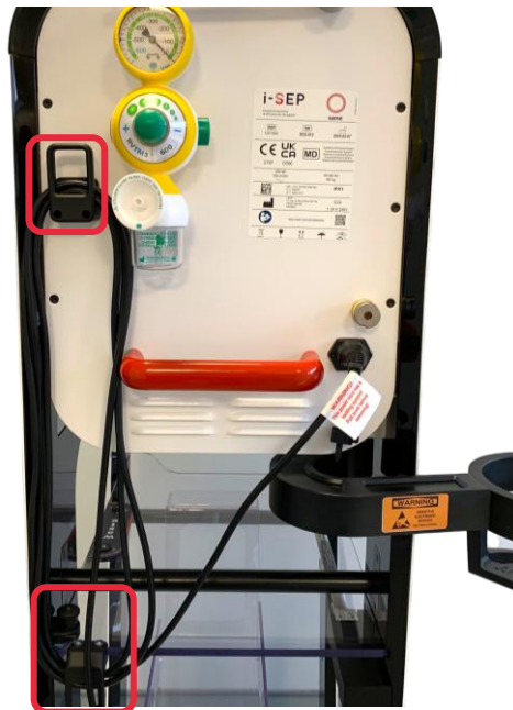
Figure 30: Cleats used to store the power cable
