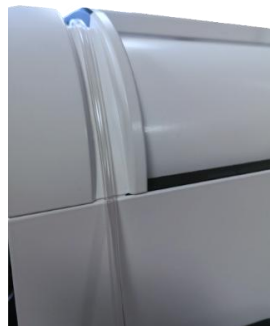
Figure 84: Insertion of the Reinfusion Line in the line guide
