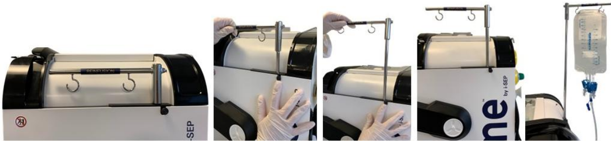
Figure 83: Reinfusion Bag installation
