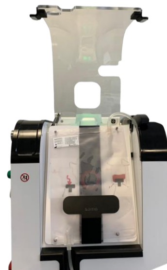
Figure 58: Treatment Bag installation
