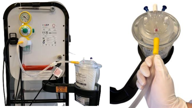
Figure 93: Aspiration vacuum installation
