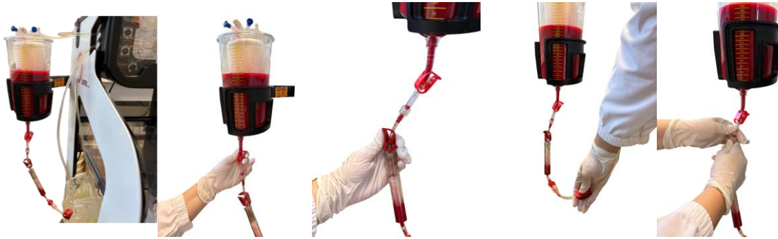
Figure 140: Changing the Micro-aggregates Chamber 1/2
