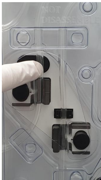
Figure 65: Pressure sensor installation
