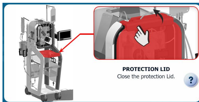
Figure 89: Closed protection lid installation screen
