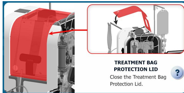
Figure 60: Closure of the treatment bag protection lid
