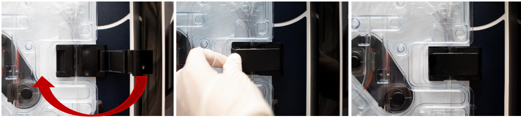
Figure 72: Closing the flap valve of the Haematocrit Reader
