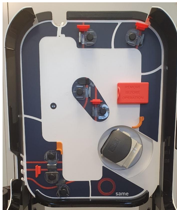
Figure 152: Covers on optical sensors
