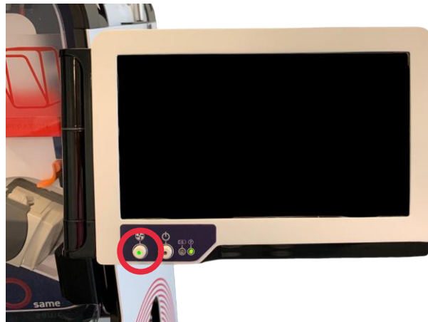
Figure 38: Pump On/Off button enabling aspiration
