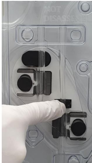
Figure 63: Fibre IN sensor tubing installation
