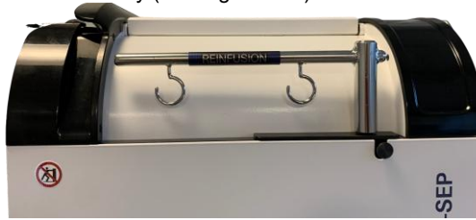
Figure 161: Stem lowered and stowed
