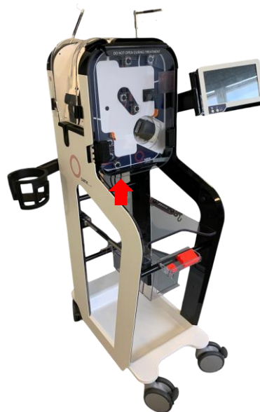
Figure 28: Position of the barcode reader and Data-Matrix
