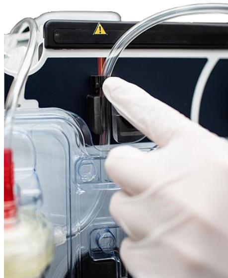
Figure 78: Waste sensor tubing installation
