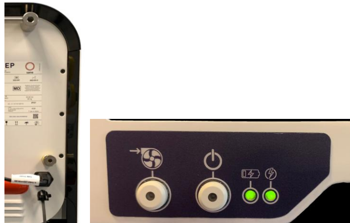
Figure 151: Connecting the ATS to power
