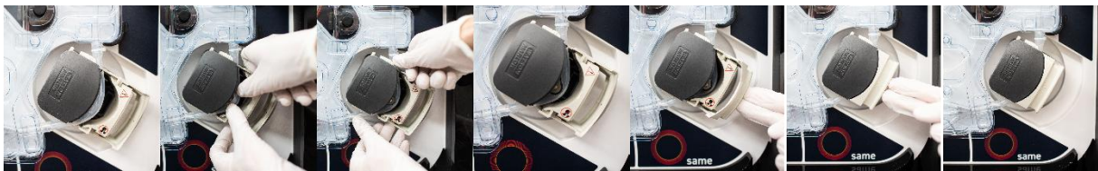
Figure 67: Tube installation in the peristaltic pump
