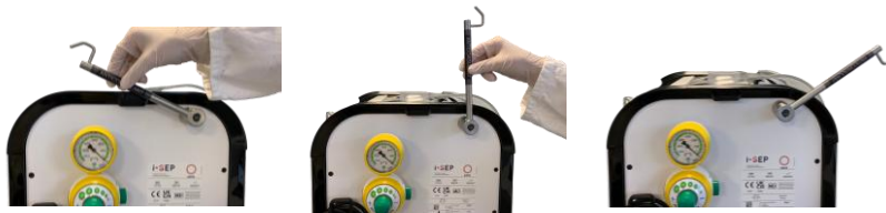
Figure 94: Anticoagulant solution holder
