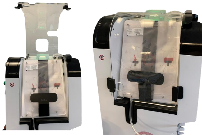
Figure 61: Closed and open Treatment Bag protection lid
