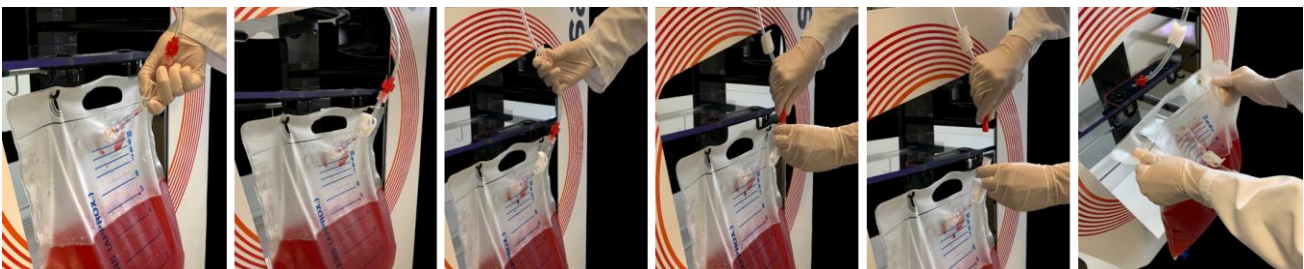
Figure 4: Replacement of the BW1000 i-SEP waste bag
