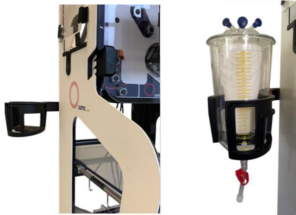
Figur 67: Installation af reservoir
